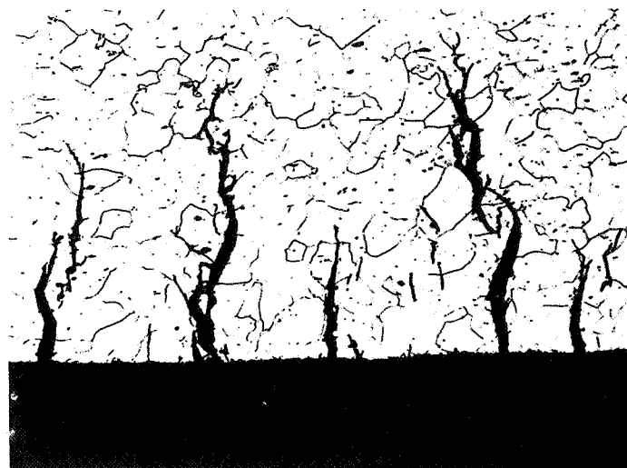
Figure 2. Transcrystalline cracking produced in Vetrocoke solution at 130°C.
